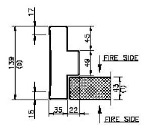
2 hours 2 Criteria Fire Rated Door, is fabricated for two hours and two criteria performance in Stability and Integrity as per BS 476 PART 22 AND IS 3614 PART II.
