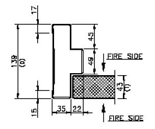
2 hours 2 Criteria Fire Rated Door, is fabricated for two hours and two criteria performance in Stability and Integrity as per BS 476 PART 22 AND IS 3614 PART II.
