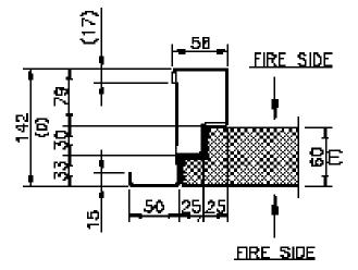
2 hours 3 Criteria Fire Rated Door, fabricated for two hours and three criteria performance in Stability, Integrity and Insulation as per BS 476 Part 22 and IS 3614 Part II, in both directions .
